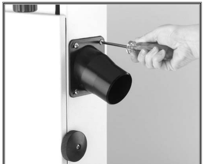
Figure 19. Installing dust port.
